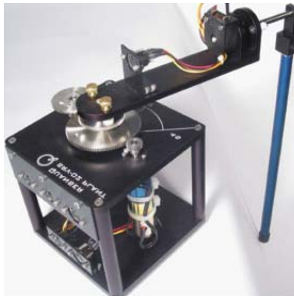
Figure 3.1 Inverted pendulum coupled to SRV02 Servomotor in the high gear ratio
